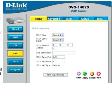
STUN is useful if you need to use the DVG-1402S behind a modem or router that provides the connection to your ISP and then to the Internet and does not support symetric NAT. You will need access to a STUN server on the Internet and its IP address to use STUN on the DVG-1402S.
